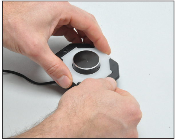
Press the acrylic panel into the face of the 1795 Rotary Control Assembly.
