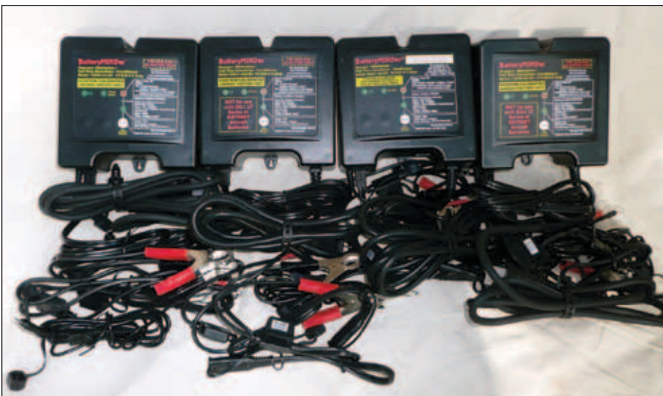
VDC BatteryMINDers, below, are the only models that use a temperature probe to adjust to optimum voltage, left.
