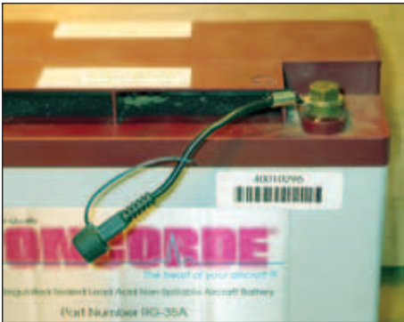
VDC BatteryMINDers, below, are the only models that use a temperature probe to adjust to optimum voltage, left.
