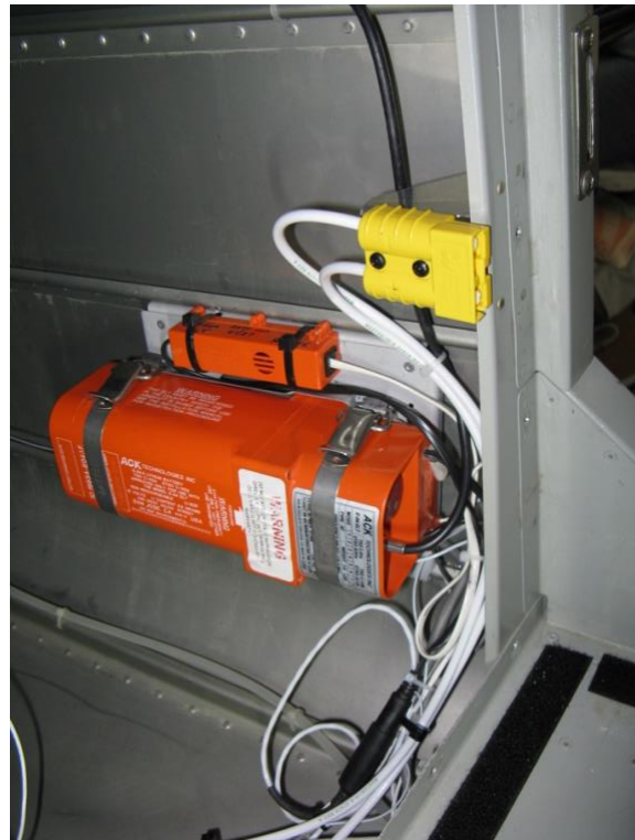
Views of the installed SB-50 plug positioned to access through the baggage closeout panel.
